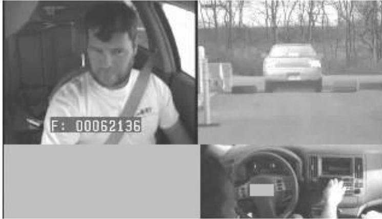
**Figure 7. Video from the Instrumented Vehicle Showing Participant Looking Up In Response to the Brake Signal**
